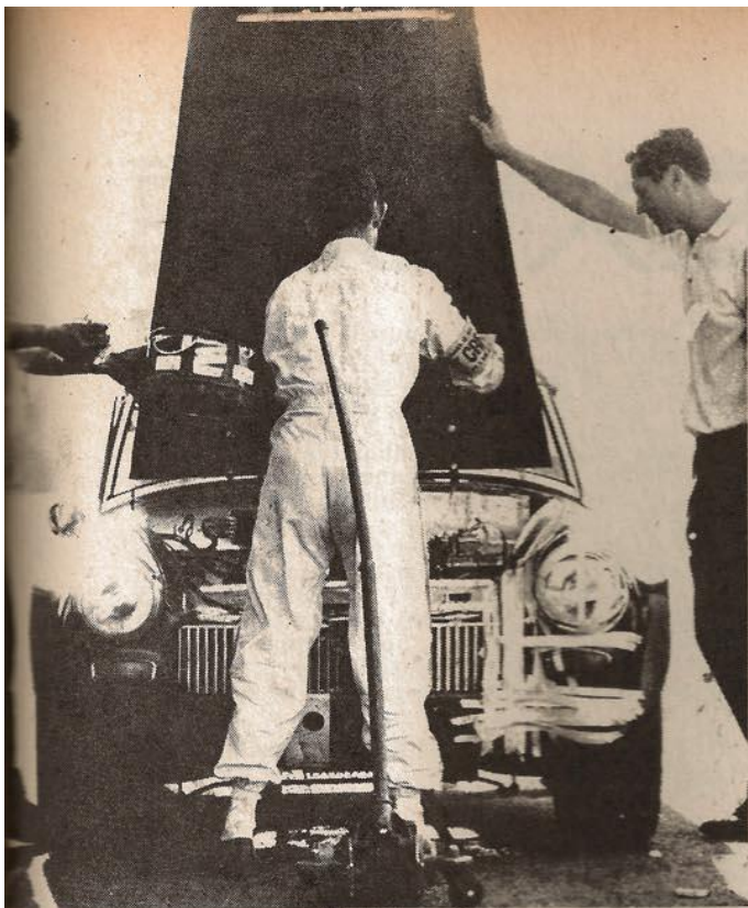
Frantic pitwork at the 12-Hour as the mechanics convert to normal wet-sump after discovering broken oil pump drive.
